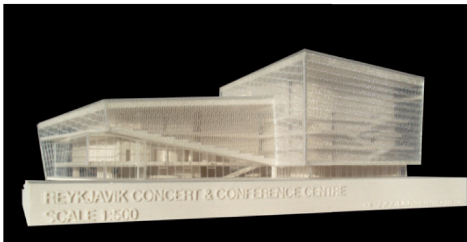
Scale model of the Reykjavik Concert and Conference Centre, made using the Z Corporation ZPrinter 450 3D printer. The interior of the Reykjavik model was printed on the Z Corp ZPrinter 450 and the skin of the building was laser cut.
